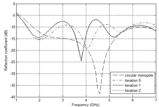
**Fig. 3 Return loss of proposed antenna structure for various iterations**
