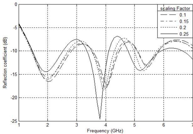
**Fig. 4 Return loss for different scaling factors**
