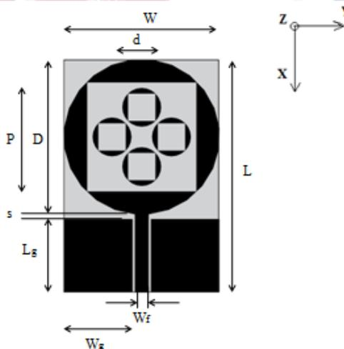
**Fig. 2 Proposed antenna structure**
