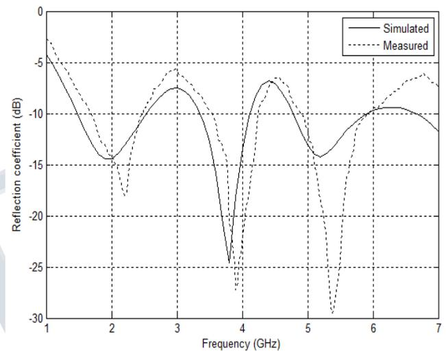
**Fig. 6 Return loss of proposed antenna**
