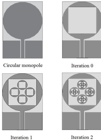
**Fig. 1 Geometrical evolution of proposed antenna**
