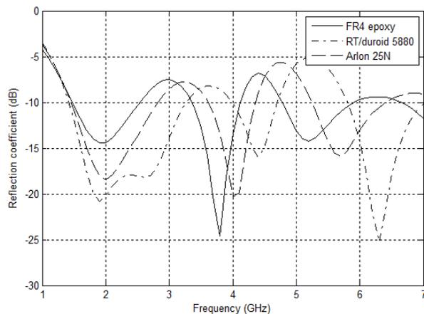
**Fig. 5 Return loss of proposed antenna on different substrates**
