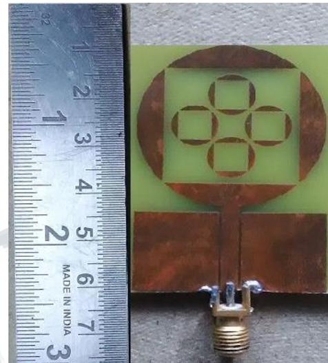
**Fig. 9 Photograph of fabricated antenna**
