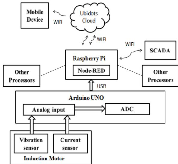
*Fig. 2 Block diagram of the proposed system*
