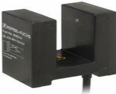
infrared light source, Not sensitive to ambient light, High switching frequency Robust and insensitive to ambient interference ,Tolerantto supply voltage variations up to 60 V DC. Sensing range 0-24mm, infrared 950 nm, and fork width 24mm.
