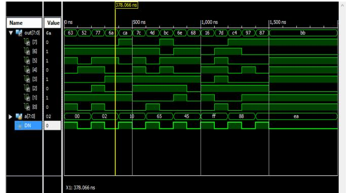
**Fig10: Simulation result of combined SubByte & InvSubByte transformations**
