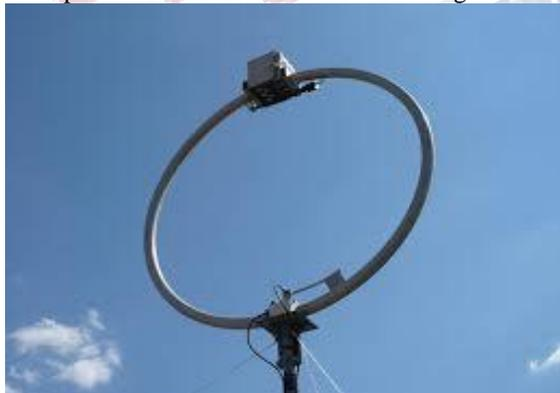
**Fig1: loop antenna**
