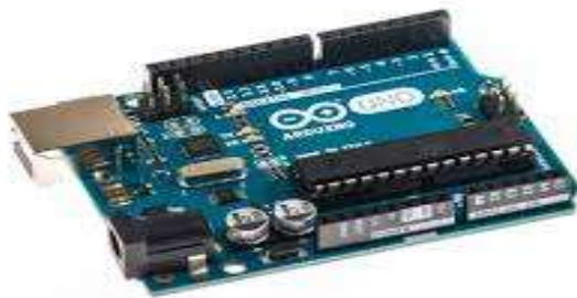
Fig.1. Arduino (ATMEGA 328P-UP)
