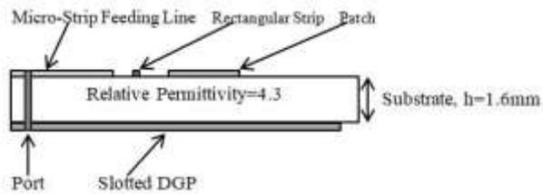
**Fig. 1 Side view geometry of OPCAC/OSS antenna**
