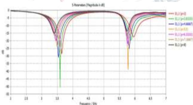
**Fig. 4 Functioning of OPCAC/OSS dual-band antenna for distinct magnitudes of W1**
