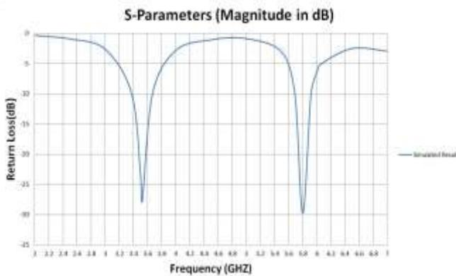
**Fig. 3 Return loss(dB) of OPCAC/OSS dual-band antenna**
