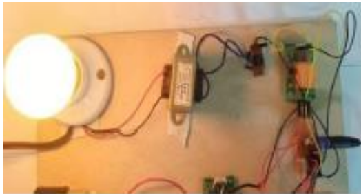
Figure 21: Set up for Power Unit Monitoring in machine ON condition
