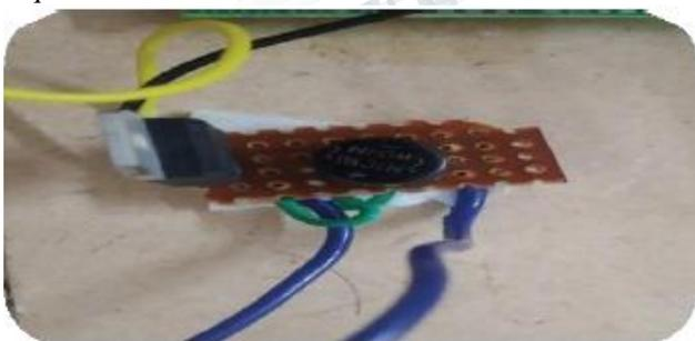
**Figure 13: Bridge Rectifier**
