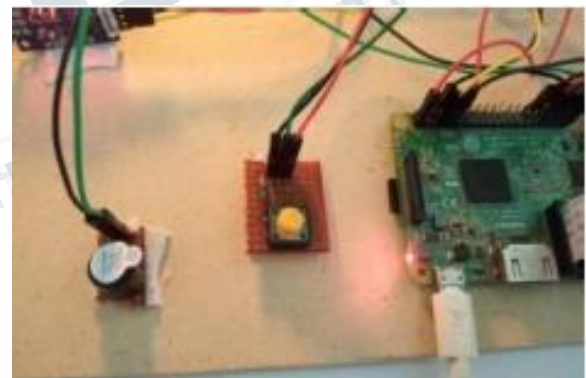
Figure 18: Setup of operator emergency alert system
