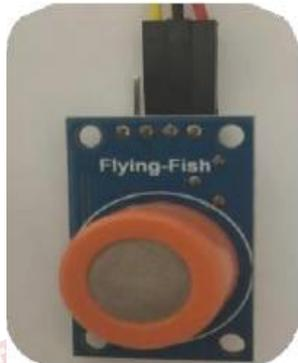
**Figure 4: Alcohol Sensor (MQ-303A)**
