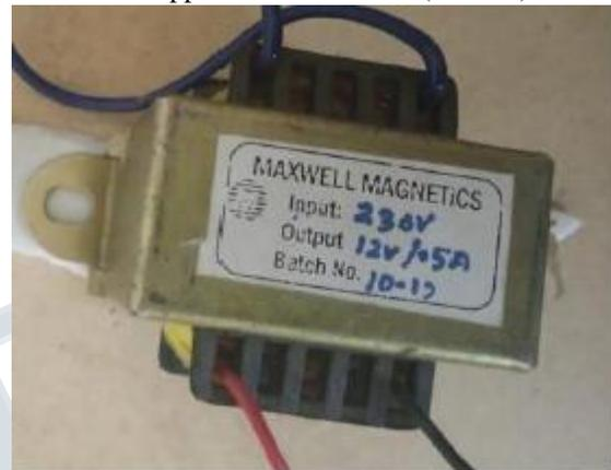
**Figure 14: Step down Transformer**
