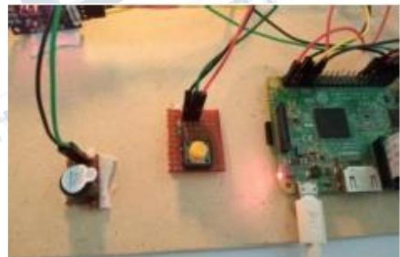
**Figure 18: Setup of operator emergency alert system**
