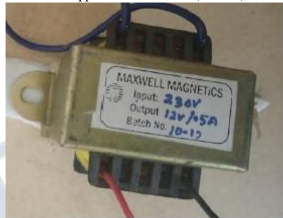
Figure 14: Step down Transformer
