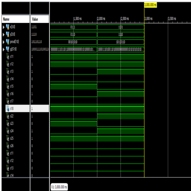
Fig. 6.2: Simulation results of existing 4x4 reversible multiplier circuit using TSG gate
