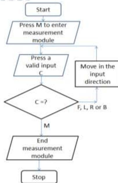
**Figure: Flow Diagram of Module 2**
