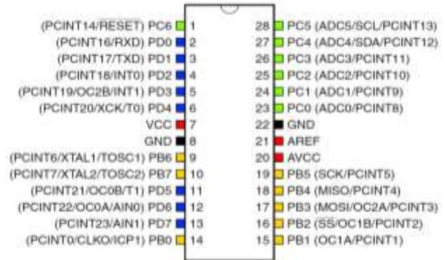
**Figure: Pin Diagram of ATmega 328P**
