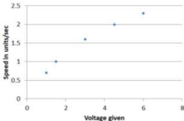
**Figure: A Graph of Robot Speed v/s Input Voltage**
