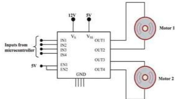
**Figure: Connection diagram of L293D motor driver to DC motors.**
