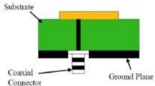
**Figure 1.3 Coaxial feed**
