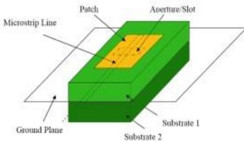
**Figure 1.4 Aperture coupled feed**
