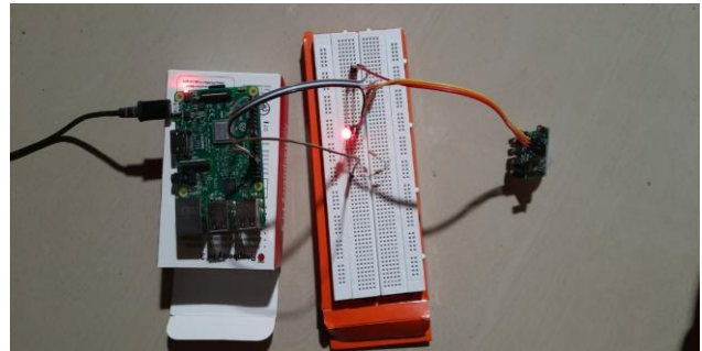
Fig 5.2 LED and PIR connected to Raspberry Pi
