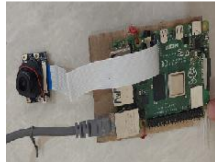
Fig.10 Interfacing of Camera to Raspberry Pi
