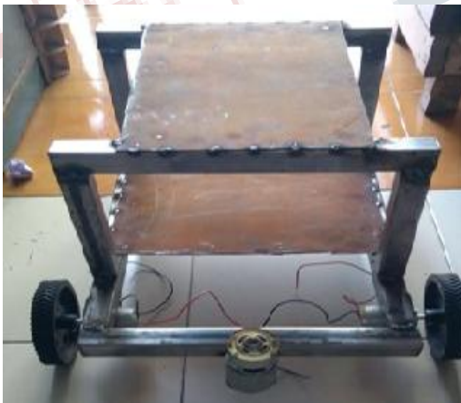
Fig.3 Mechanical Frame of Bot
