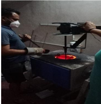
Fig 4: Aluminum Being Stirred for Effective Mixing with Reinforcement
