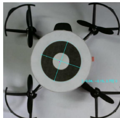
Figure 2: WhyCon Marker Detection
