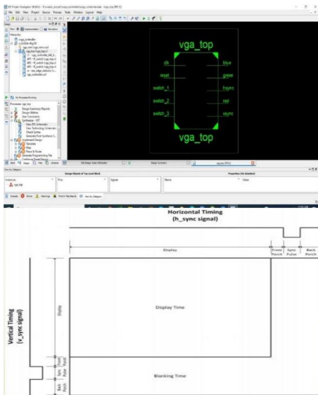
Figure 4: Top Module of VGA simulation timing
