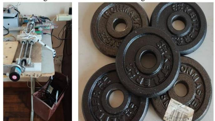
Fig. 3. Basket tied to the slider (left) where the weights (right) are placed.
