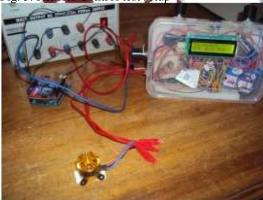
Fig. 6: LDC motor no load test
