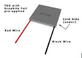
(1) Where, S is thermo power/Seebeck Coefficient of a material. The concept of thermo generators is to have two plates (one hot and other cool) creating a temperature difference having different material on both, to give a high difference in thermo power, then the Vout may be a useful amount with the high temperature difference we can get around and away from car engine
