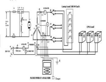
Fig[2] Experimental setup for analysis
