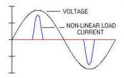
Fig[1] Waveform with non linear load A.Experimental set up
