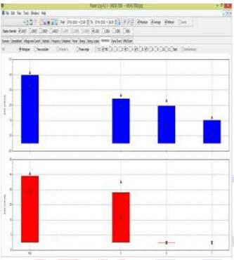
Fig[3] Observed Waveforms from fluke meter For non linear loads
