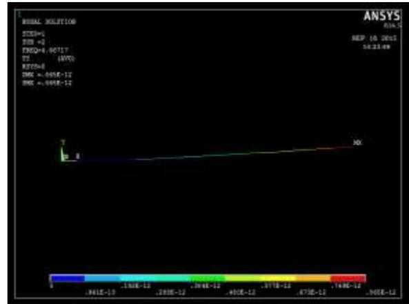
Figure 5.2: Deflection for frequency 4.667Hz
