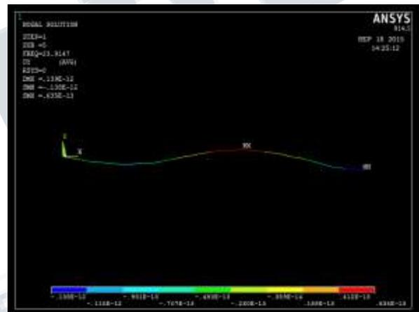
Fig. 5.3: Deflection for frequency 23.914Hz
