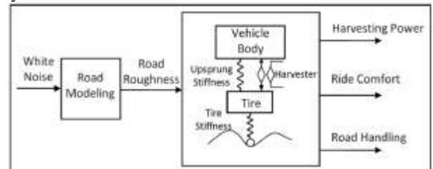
Fig. 2.1: Integrated road-vehicle harvesting model
