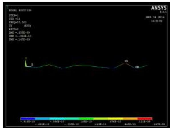
Fig. 5.4: Deflection for frequency 57.583Hz
