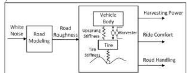
Fig. 2.1: Integrated road-vehicle harvesting model
