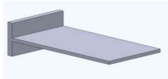
Fig. 5.1: Cantilever beam
