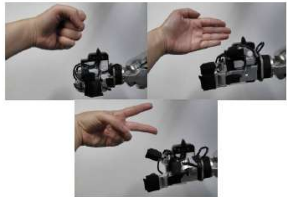
Figure 1. Example rock-paper-scissors gestures between the HRP-2 and a human (upper left: rock; upper right: paper; bottom: scissors)
