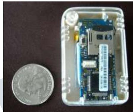
Fig. 1. The SHIMMER wearable sensor platform. SHIMMER incorporates a TI MSP430 processor, a CC2420 IEEE 802.15.4 radio, a triaxial accelerometer, and a rechargeable Li-polymer battery. The platform also includes
