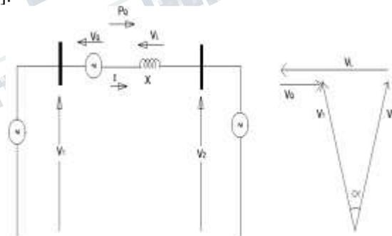
**Fig.2. The conventional two-machine system employing SSSC and related phasor diagram**
