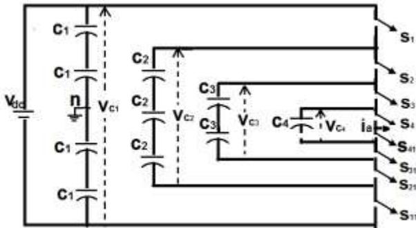
**Fig.3. Arrangement of capacitors in one phase FCMLI**
