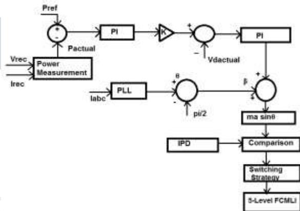
Fig.8. Control Logic of 5-level FCMLI
