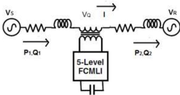
Fig.6. FCMLI connected to transmission line.
