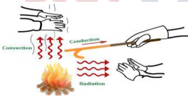
Figure 1: Schematic of modes of heat transfer.
