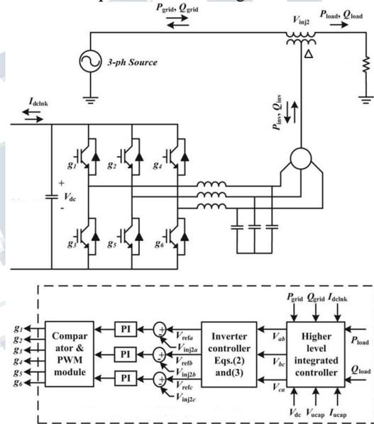
**Fig 2. Schematic diagram of three-phase series inverter and its controller**
