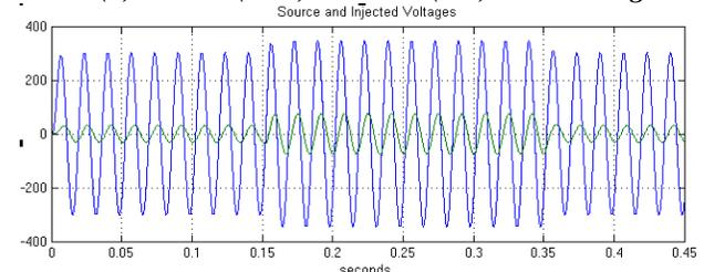
(e) Waveforms of Source(blue) and Injected(green) Voltages
