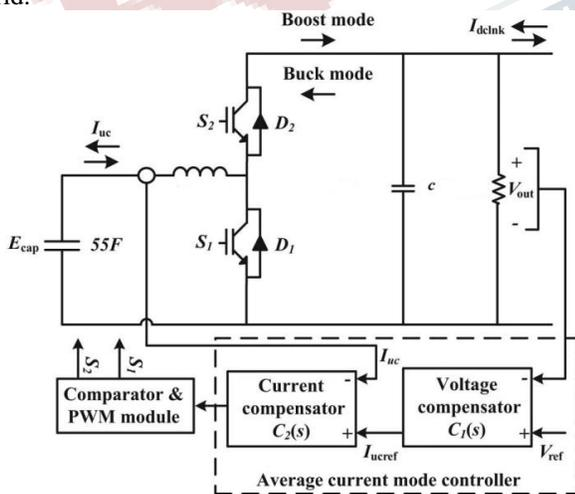
Fig. 3. Bi-directional dc-dc converter and its controller.
