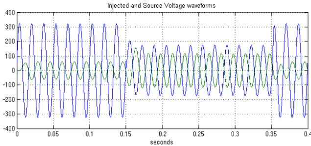
(e) Waveforms of Source(blue) and Injected(green) Voltages
