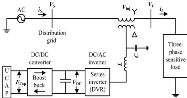
**Fig. 1. Single Line Diagram of DVR with UCAP based energy storage.**
