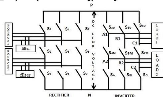
Fig. 1. Dual input Dual output indirect matrix converter
