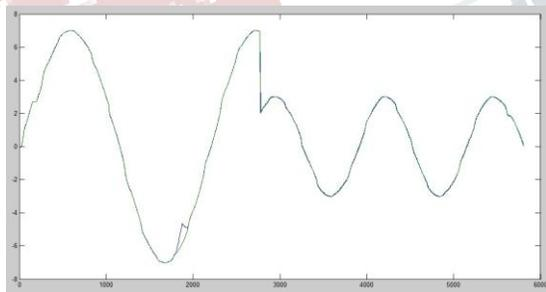
**Fig.9 Step Response for upper load Predictive Controller**
