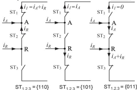
Fig.2. Three equivalent circuits for leg one of the Nine switch converter
