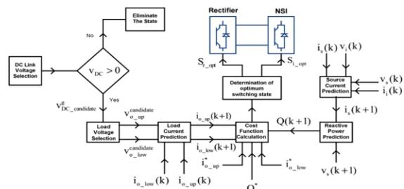
**Figure 3. Model Predictive Control Scheme for Dual Output Indirect Matrix Converter**
