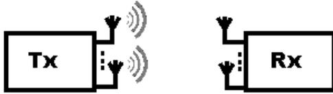
In order to be able to benefit from MIMO fully it is necessary to be able to utilise coding on the channels to separate the data from different paths. This requires processing, but provides additional channel robustness / data throughput capacity.
