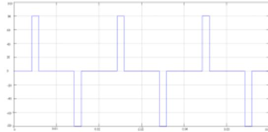
**(d) Output waveform switching angles of inverter bridge3**
