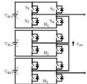
**Fig 1. Cascaded h-bridge 7-level inverter**
