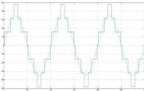
**(a) Final output waveform from the inverter**
