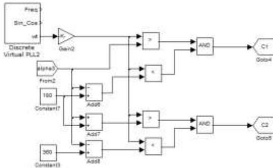
**Fig 7. Switching angles for  $H_3$**
