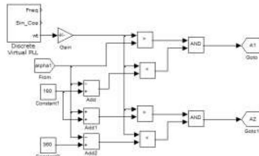
Fig 5. Switching angles for  $H_1$
