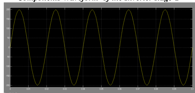
Fig. 9 : Simulink Output display of Harmonic Components Waveform of the Inverter of Stage-2, after filtered O/P
