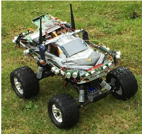
Fig. 9: The Brookes “Meanderer” vehicle duplicates the primary components of quad bicycle: camera, correspondence interface and focal control unit. It is for the most part utilized for indoor testing. The likelihood of extending the quad bicycle correspondence to a specially appointed system with at least one “Wanderers” is likewise considered.
