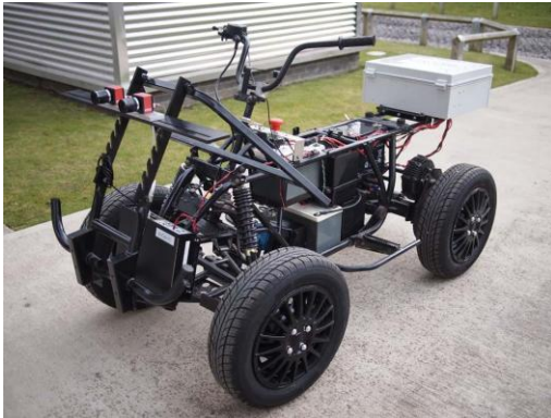
Fig. 1: The Brookes Intelligent Transport Systems Off-street off-road test vehicle proposed to resemble a 'pack donkey' that can take after a man and evade impediments.
