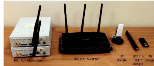
Fig. 3: Interfaces to be utilized on the OBU-ITS tested (dongles).
