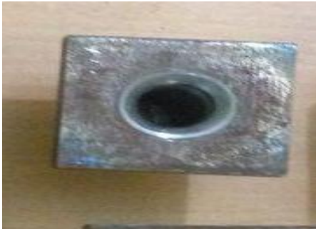
Fig.2.3. SA213 & SA387 Test sample
