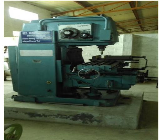
Fig 2.1 FWTPET machine (Developed In-house)
