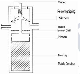
Fig : Mercury based pressure relief Valve
