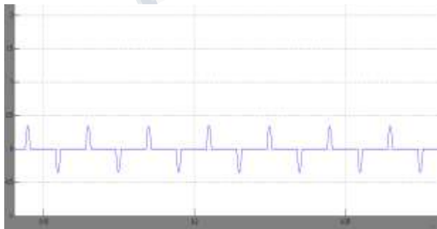
Fig 4(a) Input current of boost converter
