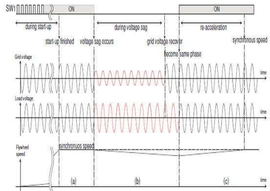
Figure 2: Operation chart of the inverter-less voltage sag compensator. (a) is idling mode and (b) is protection mode, and (c) is re-acceleration and idling mode.
