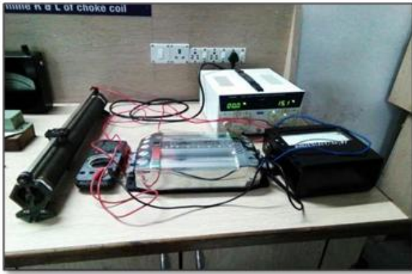
Figure 6. Hybrid super-capacitor evaluation station
