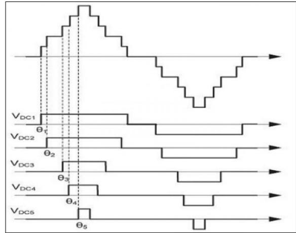
**Fig. 2 Output waveform of Eleven level inverter**
