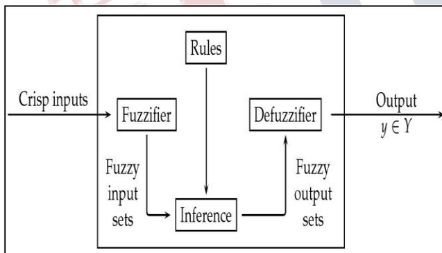
Fig.3 Block Diagram of Fuzzy logic control
