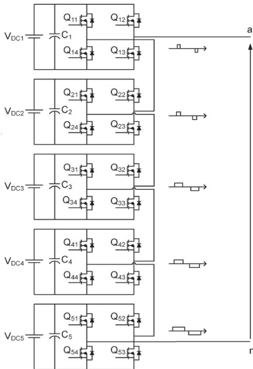
**Fig.1 Cascaded H Bridge Multilevel Inverter**
