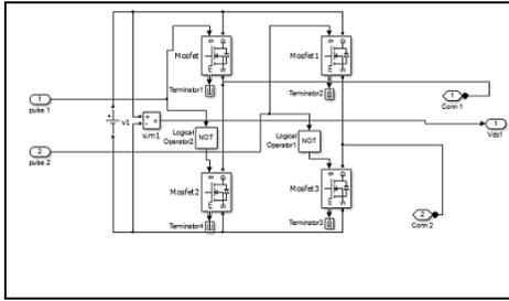
**Fig.5 Subsystem of single H Bridge**
