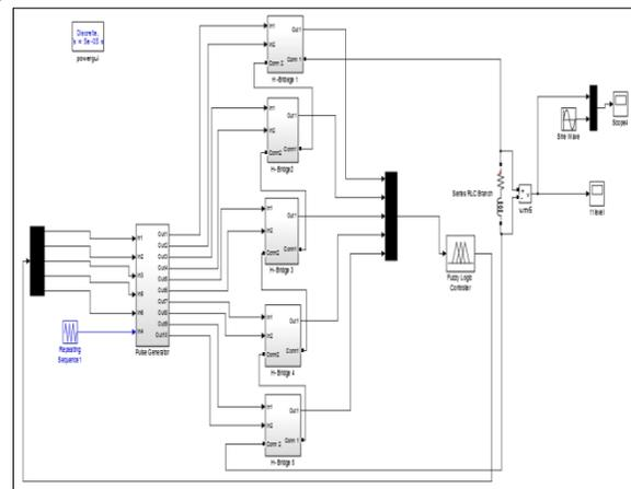
Fig. 4 Simulink diagram of the multilevel inverter with fuzzy logic
