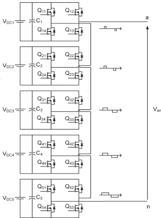
**Fig.1 Cascaded H Bridge Multilevel Inverter**
