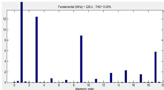
**Fig 7 FFT analysis of output voltage**
