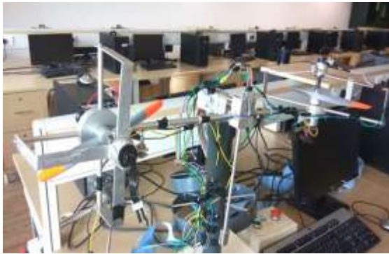
Fig. 10. TRMS System with redundant actuators
