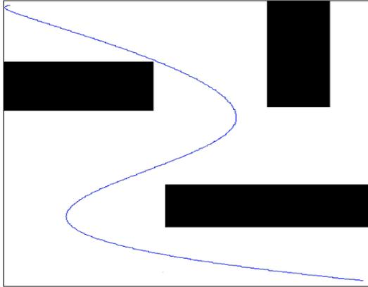
**Figure 6: robot map of a workspace; the path taken by the robot is shown in blue. This output path is obtained when genetic algorithm is used.**
