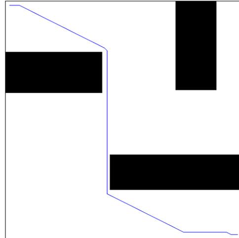
Figure 4: robot map of a workspace; the robot follows the path shown in blue; when a – star algorithm is used.
