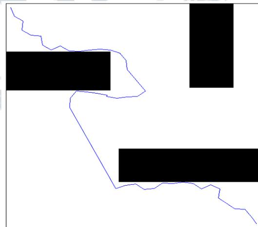
Figure 5: robot map of a workspace; the robot follows the path shown in blue; when bidirectional rrt algorithm is used.
