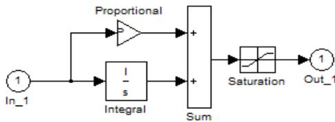
Fig. 10. Implantation the speed controller with saturation in Simulink
