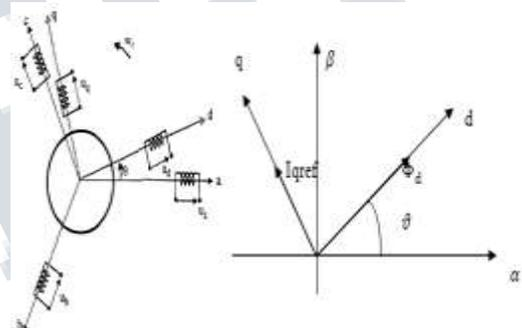
Fig. 1. Diagram representing stator winding in abc and dq frames
