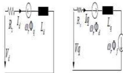
Fig. 2. Equivalent circuit of a permanent magnet synchronous motor in the dq frame
