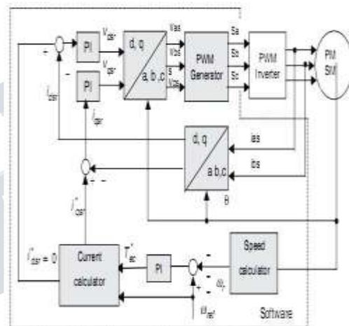
**Fig. 4. Speed control principal of a PMSM**
