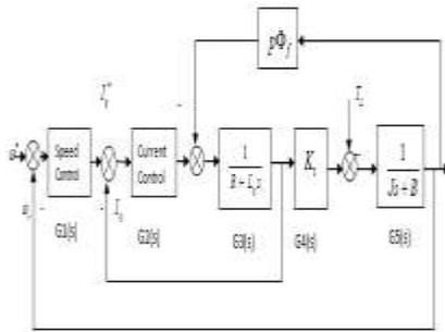
Fig. 9. Bloc diagram of a speed controlled PMSM drive
