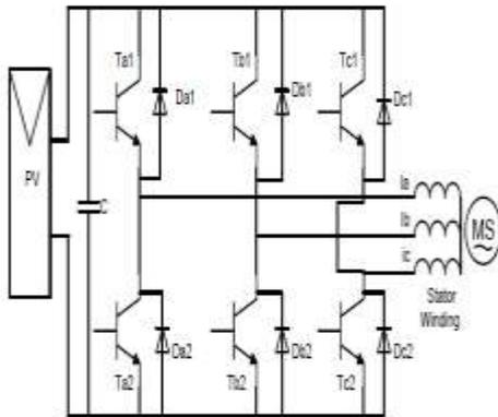
Fig. 5. PMSM supply using voltage inverter
