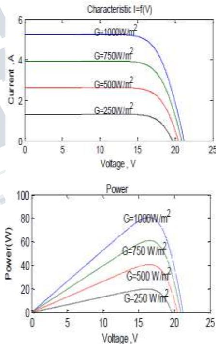
Fig. 8. Characteristics of the power function of the current and the voltage
