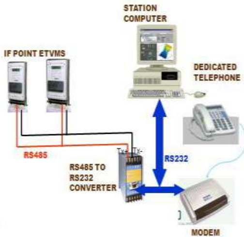
Fig.6.3.3. Connection of IF point at substation
