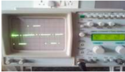
Fig 6: Inverter ac output at load of inverter circuit
