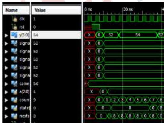
Fig4. Sensor A=4, green signal ON state
