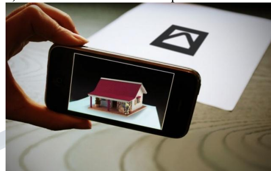
Fig. 2 Marker transformed into „Augmented Reality“ when held in view of a camera. Output as displayed on mobile screen.
