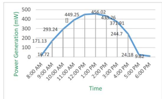
Fig. 3 Solar module readings
