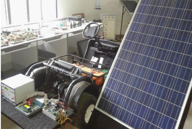
Figure.6.:Overall Test setup for Solar powered Electric vehicle
