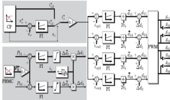
**Fig. 8. Control diagram for the fast charger with comprehensive dc power balance management.**
