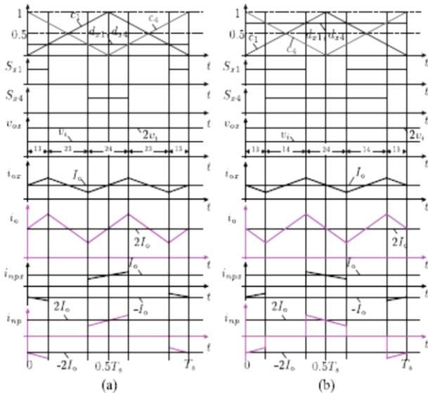
**Fig. 3. Modulation and operating principle. (a)  $d \leq 0.5$ . (b)  $d > 0.5$ .**
