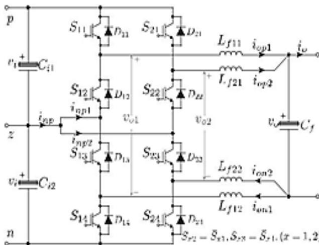
**Fig. 2. Proposed three-level dc-dc converter topology.**
