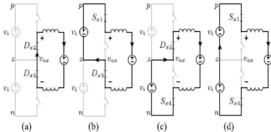
**Fig. 4. Four operating stages and their equivalent circuits. (a) 23. (b) 13. (c) 24. (d) 14.**
