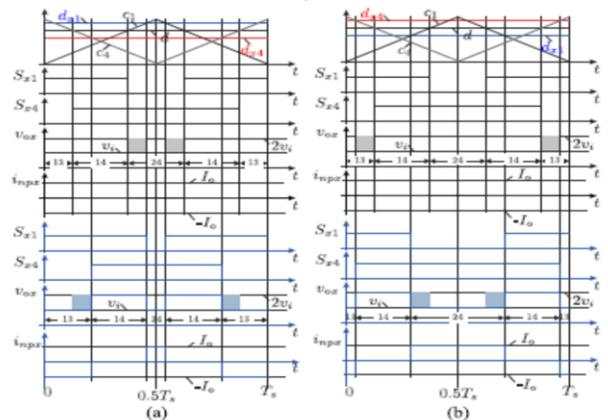
**Fig. 5. APBM principle. (a)  $dx1 > dx4$ . (b)  $dx1 < dx4$ .**
