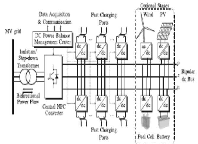
**Fig. 1. Bipolar dc bus charging station architecture**
