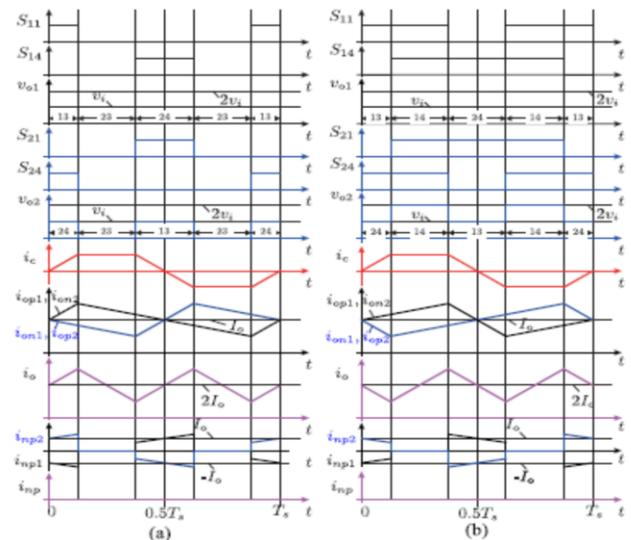
**Fig. 6. PPBM principle. (a)  $d \leq 0.5$ . (b)  $d > 0.5$ .**
