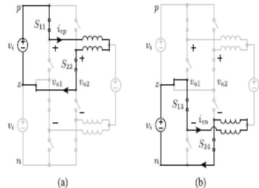
**Fig. 7. Paths for the circulating currents: (a) upper circulating current  $icp$ , (b) lower circulating current  $icn$ .**
