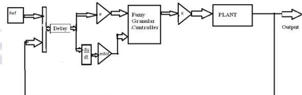
Figure 2: Representation of fuzzy logic controller [2]
