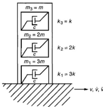
Figure 1: Representation of Dynamic system of three story building[5]
