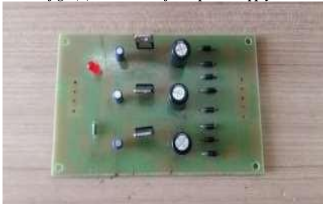
fig.a(iii) Hardware design of power supply.
