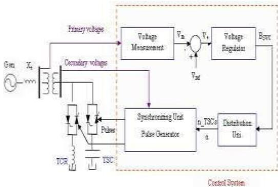
Figure 7. Control System for SVC
