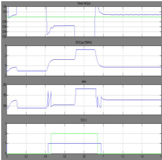
**Figure14**  $V_{meas}/V_{ref}$ , Reactive Power, No. of TSC (on/off), Firing angle  $\alpha$  and  $B_{svc}$
