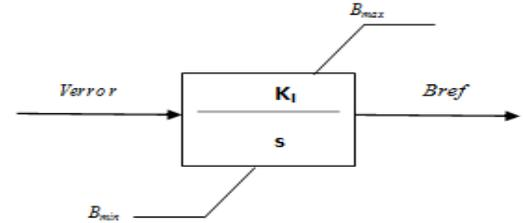
Figure 10 Voltage Regulator Model integral type.
