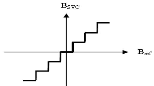
Fig.11. Distribution unit model for TSR-TSC type SVC
