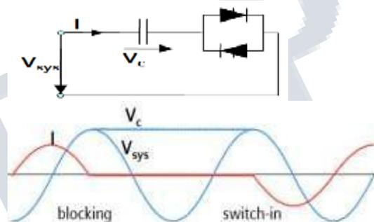
**Figure3. Basic circuit of a TSC**
