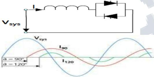
**Figure.1 Basic circuit of a TCR**
